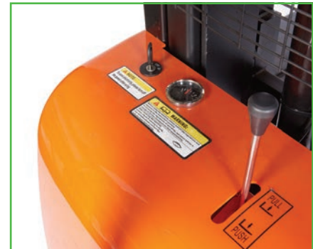
Key, Battery Life Indicator & the Fork Operating Lever on the Semi Electric Stacker
